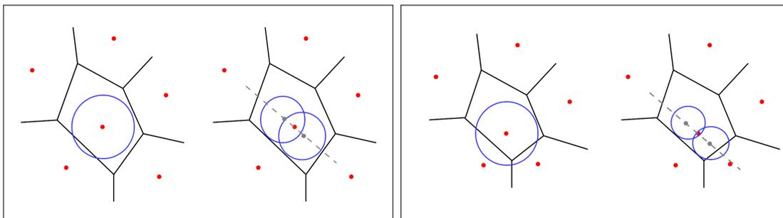
Figure 8: Schematic view of splitting algorithm. Left: Union of two circles is completely contained in the Voronoi cell. Right: Union of two circles still exceeds the Voronoi cell.
