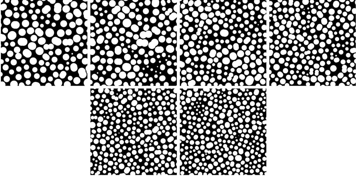
Figure 18: Predictive simulations for spin coating velocities  $\tilde{v}_1 = 625\text{rpm}$ ,  $\tilde{v}_2 = 875\text{rpm}$ ,  $\tilde{v}_3 = 1250\text{rpm}$ ,  $\tilde{v}_4 = 1750\text{rpm}$ ,  $\tilde{v}_5 = 2500\text{rpm}$  and  $\tilde{v}_6 = 3500\text{rpm}$ . The depicted area is  $3.51 \times 3.51\mu\text{m}$ .
