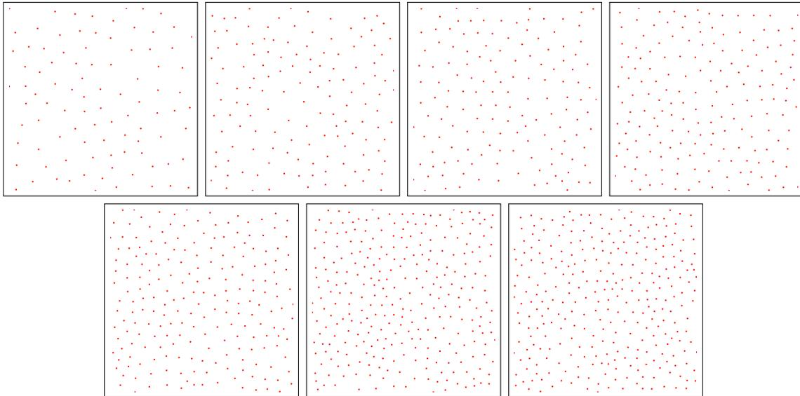
Figure 9: The centers of gravity of the particles generated by the stochastic model. Spin coating velocities from top left to bottom right:  $v_1 = 500\text{rpm}$ ,  $v_2 = 750\text{rpm}$ ,  $v_3 = 1000\text{rpm}$ ,  $v_4 = 1500\text{rpm}$ ,  $v_5 = 2000\text{rpm}$ ,  $v_6 = 3000\text{rpm}$  and  $v_7 = 4000\text{rpm}$ . The depicted area is  $3.51 \times 3.51\mu\text{m}$ .
