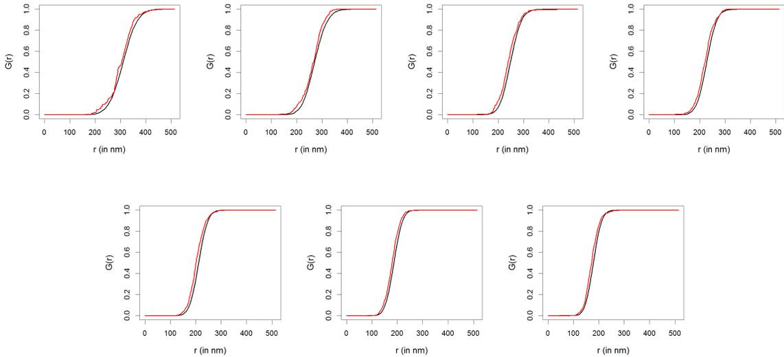
Figure 11: Nearest neighbor distance distribution function,  $G$ . Red: Experimental data. Black: Stochastic model. Spin coating velocities from top left to bottom right:  $v_1 = 500\text{rpm}$ ,  $v_2 = 750\text{rpm}$ ,  $v_3 = 1000\text{rpm}$ ,  $v_4 = 1500\text{rpm}$ ,  $v_5 = 2000\text{rpm}$ ,  $v_6 = 3000\text{rpm}$  and  $v_7 = 4000\text{rpm}$ .
