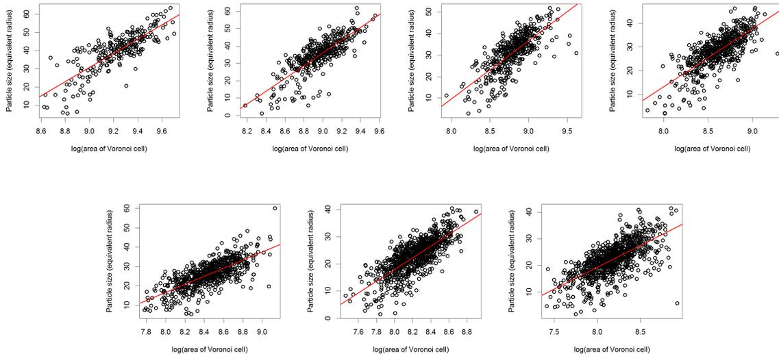
Figure 7: The equivalent radii of the particles plotted against the logarithms of the areas of the corresponding Voronoi cells, with lines of best fit shown. Spin coating velocities from top left to bottom right:  $v_1 = 500\text{rpm}$ ,  $v_2 = 750\text{rpm}$ ,  $v_3 = 1000\text{rpm}$ ,  $v_4 = 1500\text{rpm}$ ,  $v_5 = 2000\text{rpm}$ ,  $v_6 = 3000\text{rpm}$  and  $v_7 = 4000\text{rpm}$ .
