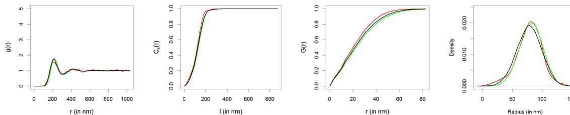
Figure 21: Characteristics of experimental and simulated morphologies corresponding to a spin velocity of 3000rpm. Red: Experimental data set. Black: Stochastic model with parameters fitted to the whole data set. Green: Stochastic model fitted without the data for  $v_6 = 3000$ rpm. From left to right: Pair correlation function, chord length distribution in  $x$ -direction, spherical contact distance distribution from polymer-rich phase to particles and size distribution of particles.
