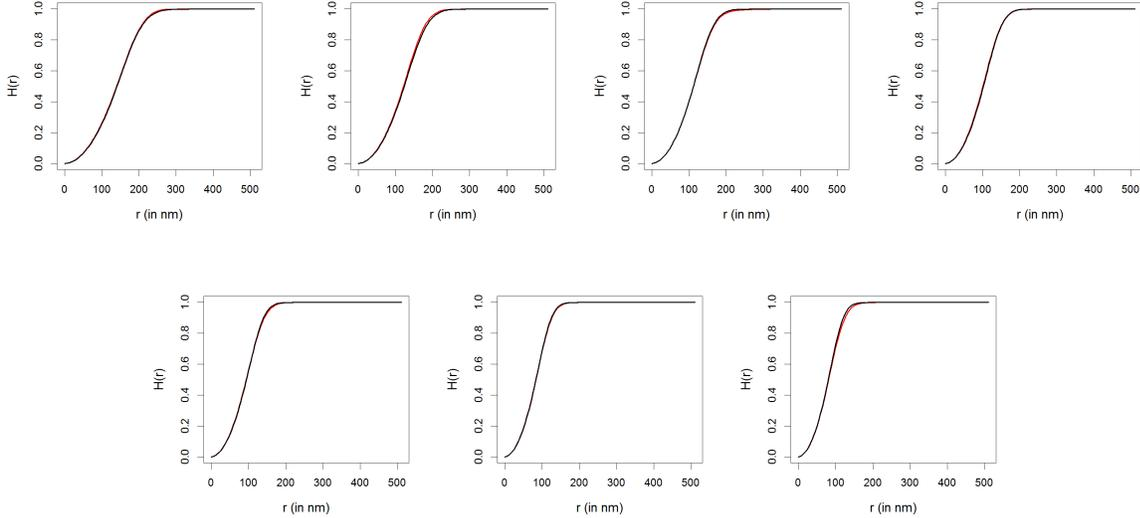
Figure 12: Spherical contact distance distribution function,  $H$ . Red: Experimental data. Black: Stochastic model. Spin coating velocities from top left to bottom right:  $v_1 = 500\text{rpm}$ ,  $v_2 = 750\text{rpm}$ ,  $v_3 = 1000\text{rpm}$ ,  $v_4 = 1500\text{rpm}$ ,  $v_5 = 2000\text{rpm}$ ,  $v_6 = 3000\text{rpm}$  and  $v_7 = 4000\text{rpm}$ .
