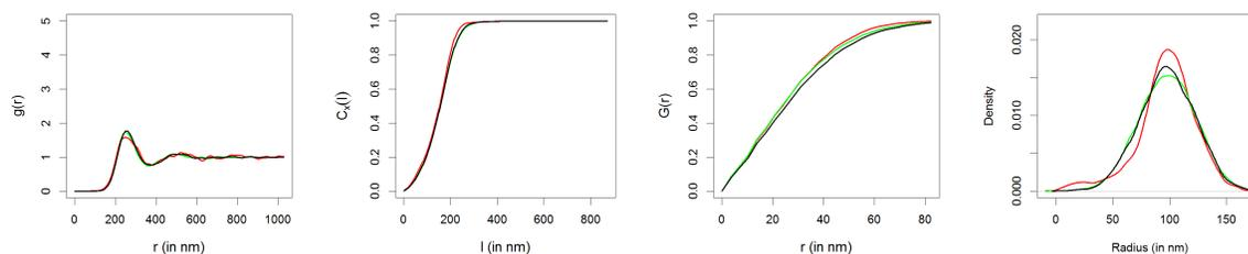
Figure 20: Characteristics of experimental and simulated morphologies corresponding to a spin velocity of 1500rpm. Red: Experimental data set. Black: Stochastic model with parameters fitted to the whole data set. Green: Stochastic model fitted without the data for  $v_4 = 1500$ rpm. From left to right: Pair correlation function, chord length distribution in  $x$ -direction, spherical contact distance distribution from polymer to particle and size distribution of particles.
