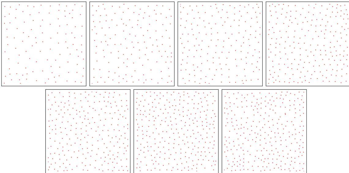
Figure 3: The centers of gravity of the particles shown in Figures 1 and 2. Spin coating velocities from top left to bottom right:  $v_1 = 500\text{rpm}$ ,  $v_2 = 750\text{rpm}$ ,  $v_3 = 1000\text{rpm}$ ,  $v_4 = 1500\text{rpm}$ ,  $v_5 = 2000\text{rpm}$ ,  $v_6 = 3000\text{rpm}$  and  $v_7 = 4000\text{rpm}$ . The depicted area is  $3.51 \times 3.51\mu\text{m}$ .
