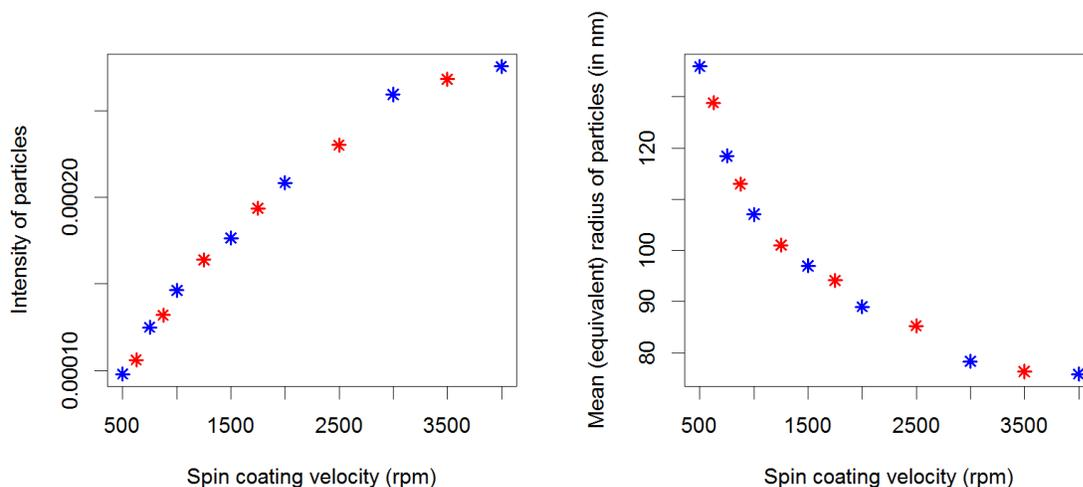
Figure 19: Intensity and mean size of particles in relation to spin coating velocities. Blue: Experimental data. Red: Predictive simulations.
