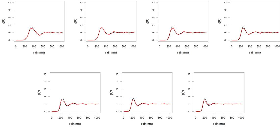
Figure 10: Pair correlation function,  $g$ . Red: Experimental data. Black: Stochastic model. Spin coating velocities from top left to bottom right:  $v_1 = 500\text{rpm}$ ,  $v_2 = 750\text{rpm}$ ,  $v_3 = 1000\text{rpm}$ ,  $v_4 = 1500\text{rpm}$ ,  $v_5 = 2000\text{rpm}$ ,  $v_6 = 3000\text{rpm}$  and  $v_7 = 4000\text{rpm}$ .
