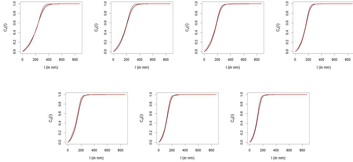
Figure 15: Chord length distribution,  $C_x$ . Red: Experimental data. Black: Stochastic model. Spin coating velocities from top left to bottom right:  $v_1 = 500\text{rpm}$ ,  $v_2 = 750\text{rpm}$ ,  $v_3 = 1000\text{rpm}$ ,  $v_4 = 1500\text{rpm}$ ,  $v_5 = 2000\text{rpm}$ ,  $v_6 = 3000\text{rpm}$  and  $v_7 = 4000\text{rpm}$ .
