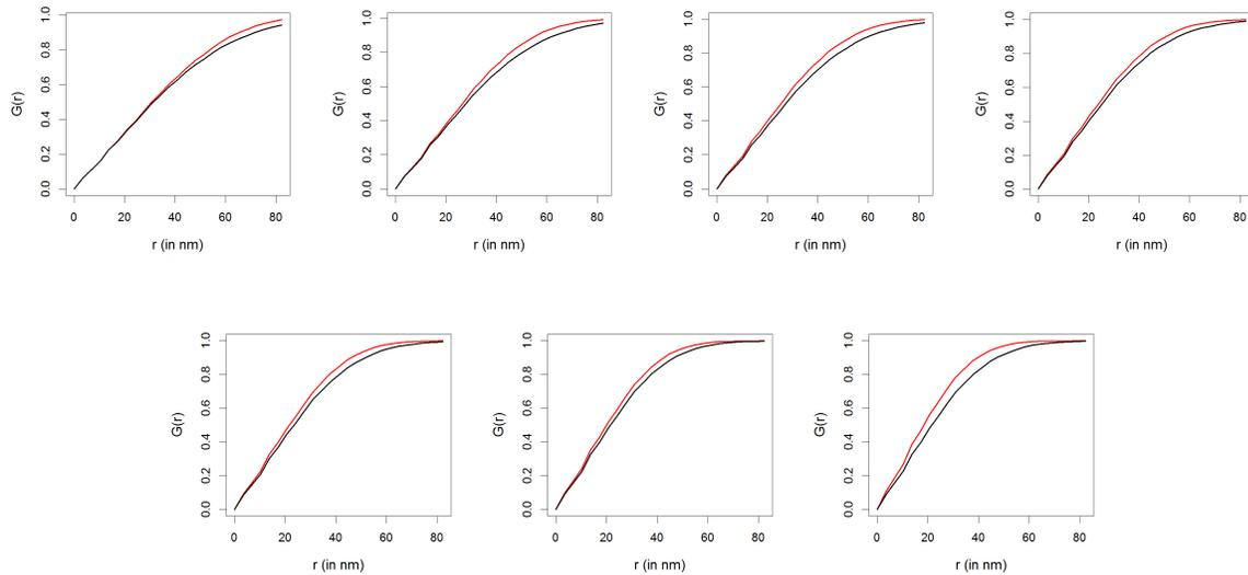
Figure 16: Spherical contact distance distributions,  $G$ , from the polymer-rich phase to the particle phase. Red: experimental data; black: stochastic model. Spin coating velocities from top left to bottom right:  $v_1 = 500\text{rpm}$ ,  $v_2 = 750\text{rpm}$ ,  $v_3 = 1000\text{rpm}$ ,  $v_4 = 1500\text{rpm}$ ,  $v_5 = 2000\text{rpm}$ ,  $v_6 = 3000\text{rpm}$  and  $v_7 = 4000\text{rpm}$ .
