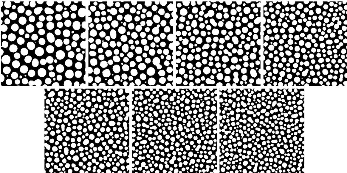
Figure 2: The binarized images corresponding to the images in Figure 1. White represents the fullerene-rich domains and black represents the polymer-rich matrix. Spin coating velocities from top left to bottom right:  $v_1 = 500\text{rpm}$ ,  $v_2 = 750\text{rpm}$ ,  $v_3 = 1000\text{rpm}$ ,  $v_4 = 1500\text{rpm}$ ,  $v_5 = 2000\text{rpm}$ ,  $v_6 = 3000\text{rpm}$  and  $v_7 = 4000\text{rpm}$ . The depicted area is  $3.51 \times 3.51\mu\text{m}$ .
