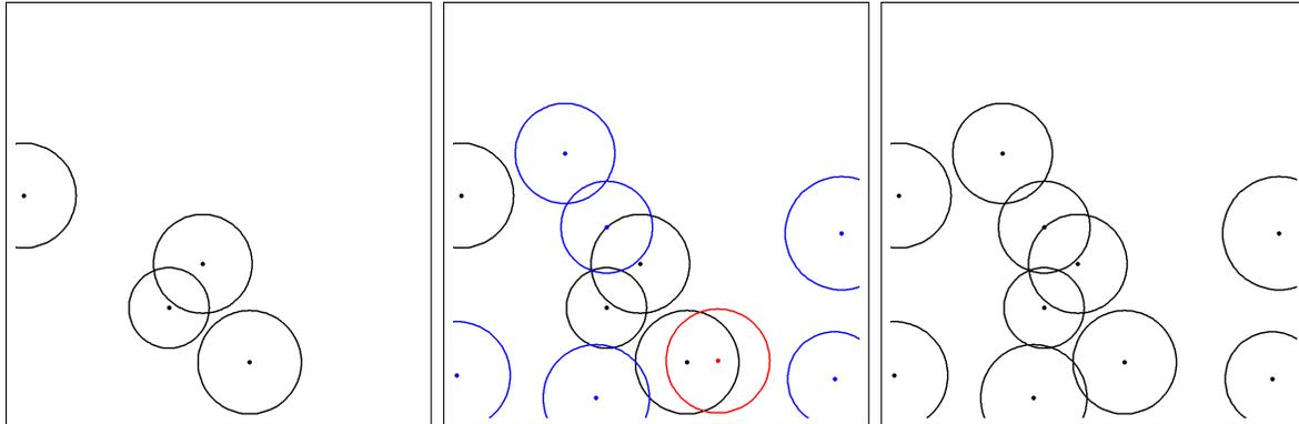
(a) Left: The first point pattern is generated. Center: The second point pattern is generated and each point is checked to make sure that it satisfies (1). The points to be added are shown in blue and those that will not are shown in red. Right: The point pattern after the points are added.
