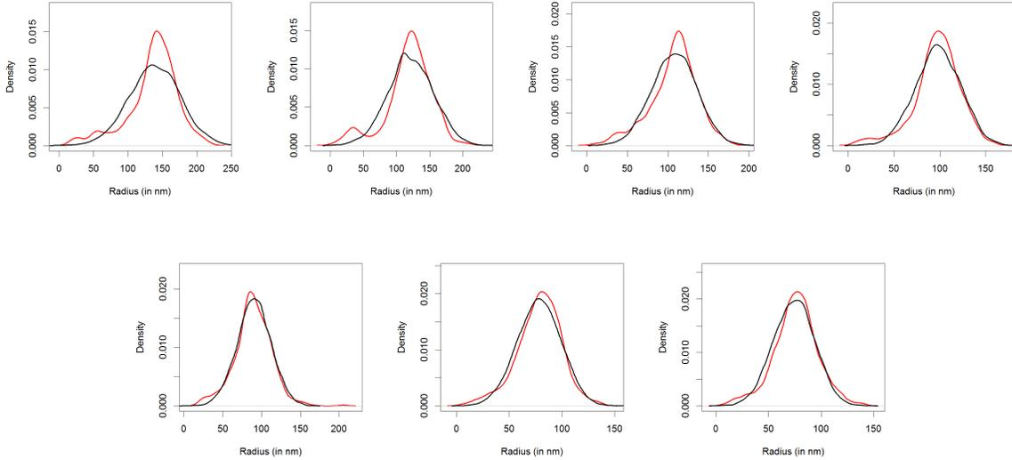
Figure 14: Particle size distribution. Red: Experimental data. Black: Stochastic model. Spin coating velocities from top left to bottom right:  $v_1 = 500\text{rpm}$ ,  $v_2 = 750\text{rpm}$ ,  $v_3 = 1000\text{rpm}$ ,  $v_4 = 1500\text{rpm}$ ,  $v_5 = 2000\text{rpm}$ ,  $v_6 = 3000\text{rpm}$  and  $v_7 = 4000\text{rpm}$ .
