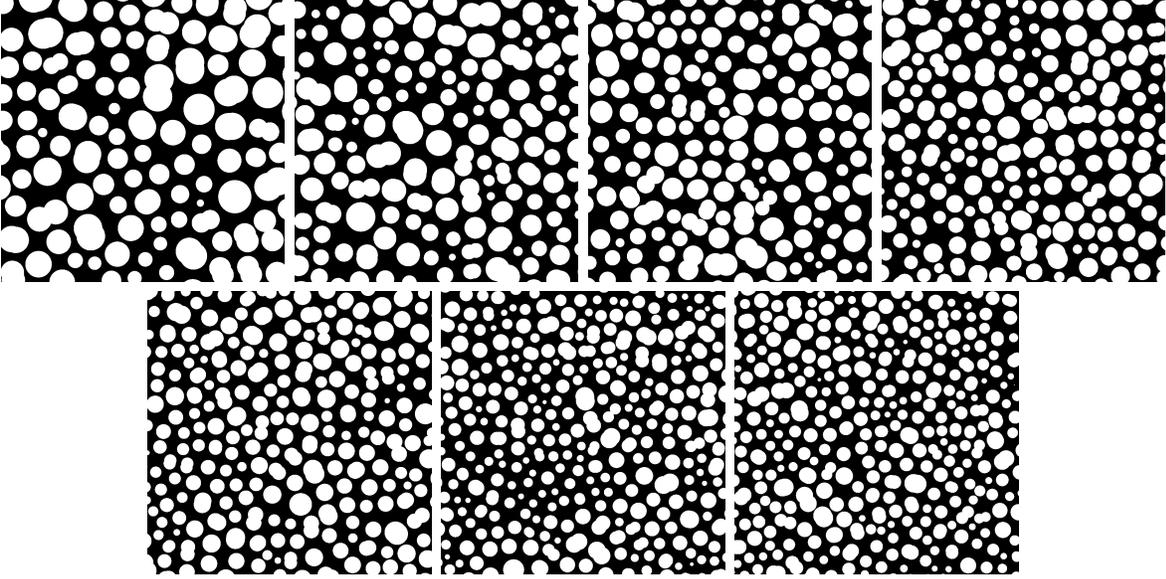
Figure 13: Realizations of the stochastic model. Spin coating velocities from top left to bottom right:  $v_1 = 500\text{rpm}$ ,  $v_2 = 750\text{rpm}$ ,  $v_3 = 1000\text{rpm}$ ,  $v_4 = 1500\text{rpm}$ ,  $v_5 = 2000\text{rpm}$ ,  $v_6 = 3000\text{rpm}$  and  $v_7 = 4000\text{rpm}$ . The depicted area is  $3.51 \times 3.51\mu\text{m}$ .
