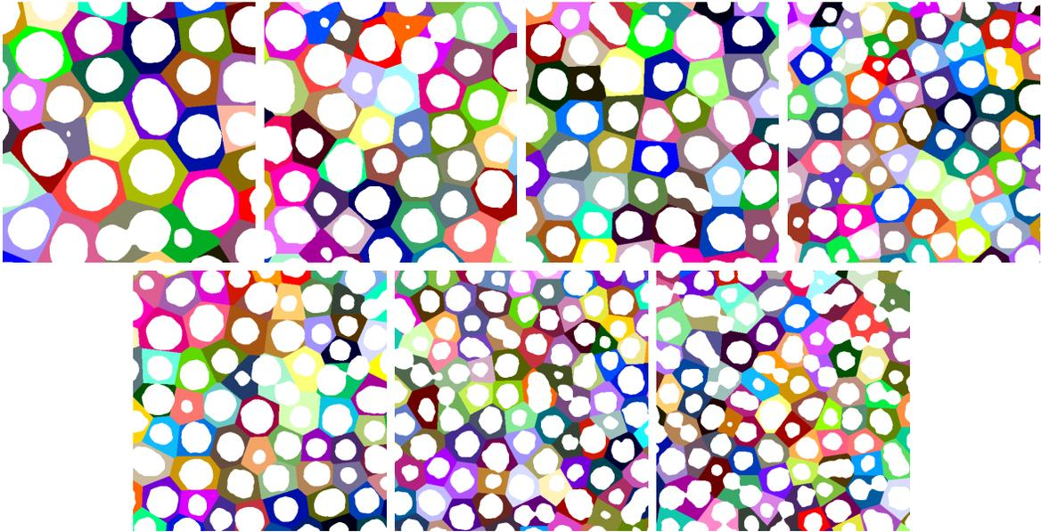
Figure 6: Voronoi tessellation on cutout of particle midpoints. Spin coating velocities from top left to bottom right:  $v_1 = 500\text{rpm}$ ,  $v_2 = 750\text{rpm}$ ,  $v_3 = 1000\text{rpm}$ ,  $v_4 = 1500\text{rpm}$ ,  $v_5 = 2000\text{rpm}$ ,  $v_6 = 3000\text{rpm}$  and  $v_7 = 4000\text{rpm}$ . The depicted area is about  $1.9 \times 1.9\mu\text{m}$ .
