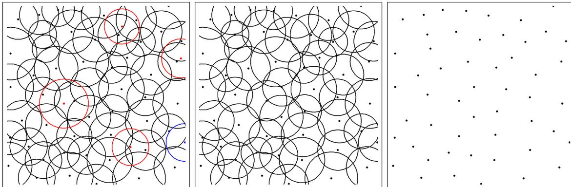
(b) Left: This procedure is continued many times. Center: We stop adding points when 99.9% of the simulation window is covered by circles. Right: The center points of the circles are kept as the particle locations.
