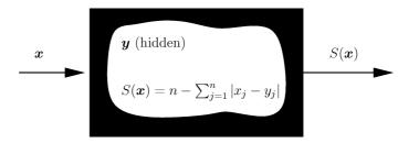
Figure 2. A black box for decoding vector y.
