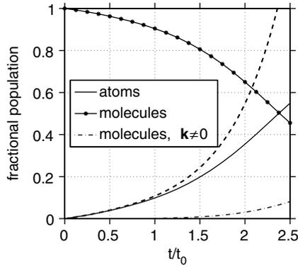
FIG. 1. Fractional population in the molecular and atomic fields,  $N_0(t)/N_0(0)$  and  $N_1(t)/2N_0(0)$ , as a function of time  $t$ . The time is in units of  $t_0=1/g=1/(\chi\sqrt{\rho_0})$ , which in this example is  $t_0=0.2$  ms. The dash-dotted line is the fraction of molecules in the noncondensate modes,  $\mathbf{k}\neq 0$ . The dashed line is the analytic result for the total atom number in the undepleted molecular field approximation.
