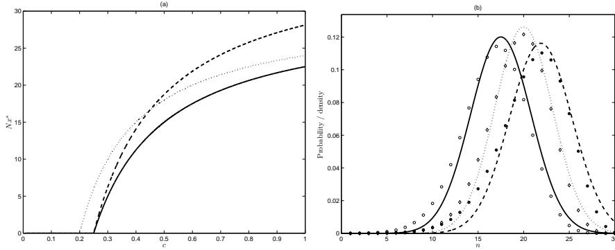
FIG 4.  $N$ -patch metapopulation model with  $N = 30$ ,  $e = 0.2$  and  $c(x) = cx$ . (a)  $x_{CE}^*$  (solid),  $x_{SIS}^*$  (dotted) and  $x_{EC}^*$  (dashed) versus  $c$ . (b) pdf of the stationary distribution of the limiting Gaussian process for the CE model (solid), the SIS model (dotted) and the EC model (dashed) with  $c = 0.6$ , together with the corresponding quasi-stationary distributions (open circles, diamonds and solid circles).
