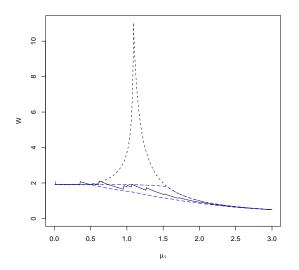
Expected transit times under user optimal policy for state-dependent routing (\_\_\_\_\_\_), and probabilistic routing (\_\_\_\_\_\_)  $\lambda = 1, \lambda_2 = 0.1, \mu_2 = 1, N = 3$  for  $0 \le \mu_1 \le 3$ .
