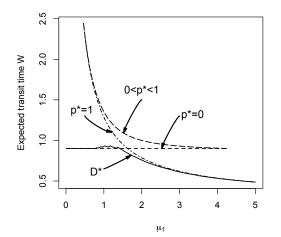
Expected transit times under user optimal policy for state-dependent routing (\_\_\_\_\_\_), and probabilistic routing (\_\_\_\_\_\_),  $\lambda_2 = 4, \lambda_1 = 3, \lambda_2 = 1, \mu_2 = 2, N_1 = N_2 = 5$  for  $0 \le \mu_1 \le 6$ . Chen, Holmes, Z(2011)
