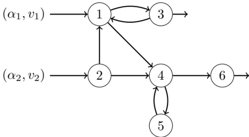
**Single-class:** Each queue has a dedicated (separate) server (all parts of brain can process in parallel)
